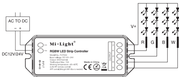
Controller connect to RGBW LED strip diagram
