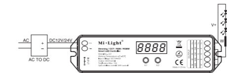
Controller connect to Single Color LED strip diagram
